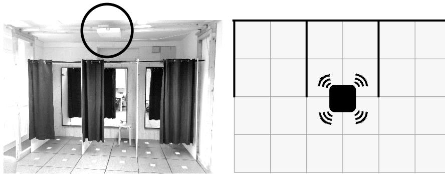
Figure 1. Test environment with ceiling-mounted RFID system and three fitting room cabins
