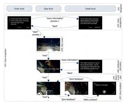
Figure 2. Screens of the smart glasses-based service support system (instantiating DP1-7)
